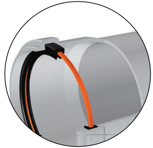
Collar interval in the installation of PVC Dublex Pipes and Fittings should be 1 m.
